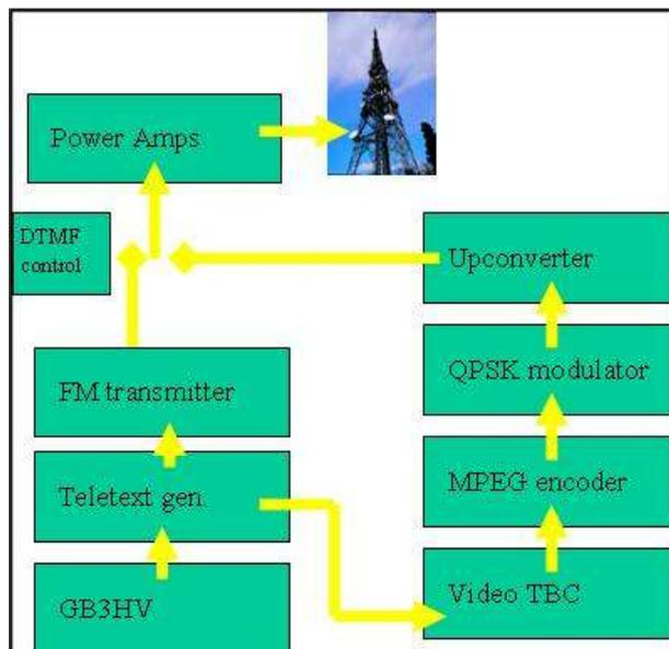
A standard amateur linear transmit up converter, designed for SSB operation, is driven by the IF output of the modulator and produces a low level signal (approx +3dBm at
