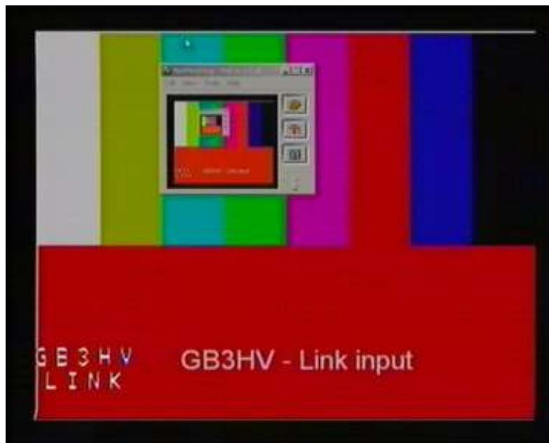
Whilst Netmeeting will automatically answer incoming calls, nothing will be displayed on the repeater output until the keeper using 432MHz telemetry input enters the correct DTMF commands to select the input. Thereby the internet input does not have any control over the repeater, although a DTMF \* received on the input will transmit a 1Khz “notification” tone for 5 seconds when GB3HV is in transmit but the selection of the input is always under local control.
